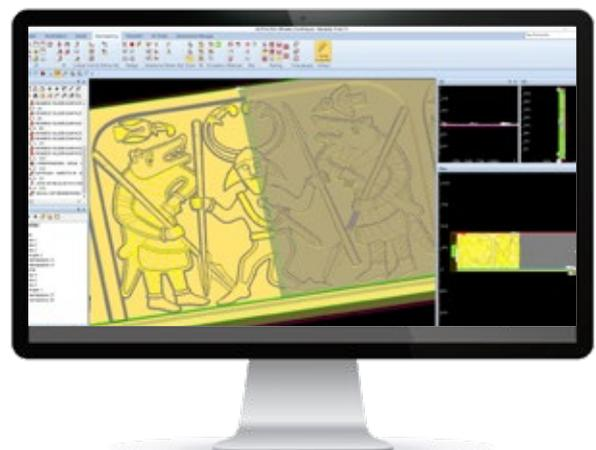
The decorations were created by the museum, based on original designs found in graves and excavations in Denmark, Sweden and Norway. Bystrup Maskinsnedkeri received them as STEP files, which were imported into ALPHACAM. The designs sank into the wood to a depth of 25mm, and were machined with small ball nose cutters, which were required to achieve the necessary detail.
